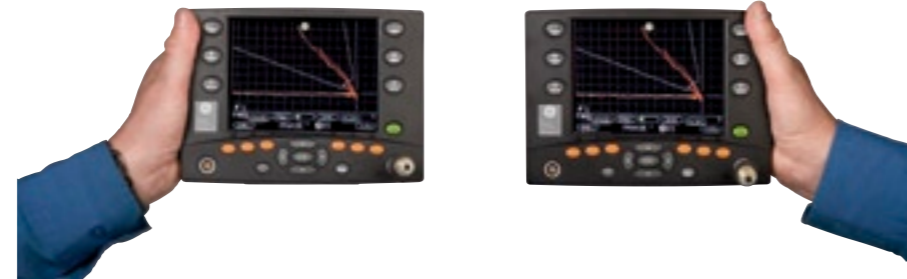
Ambidextrous: the instrument can be operated by left and right handed people with the same level of comfort. The most used key during inspection can be reached with one finger.
